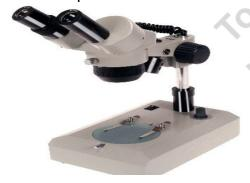
This is a light microscope. It lets you magnify images that light can pass through. Uses glass slide and cover slip.
